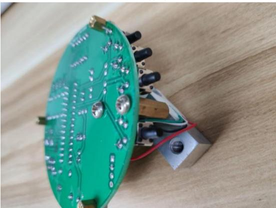
Use two long screws to fix the sensor;
